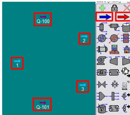
2. In order to make the simulation easy to follow, rename the material streams to feed, distillate, and bottoms. Rename the energy streams to condenser energy, and reboiler energy.
