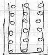
$$e_h = \frac{b_0 - 4\phi - 2c - 3\phi}{2} = 7,0 \text{ cm.}$$
