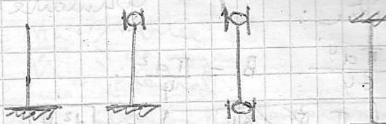
$$l_f = 2 l_0 \quad ; \quad l_f = \frac{l_0}{\sqrt{2}} \quad l_0 = \frac{l_f}{\sqrt{2}} = \frac{l_f}{2}$$
