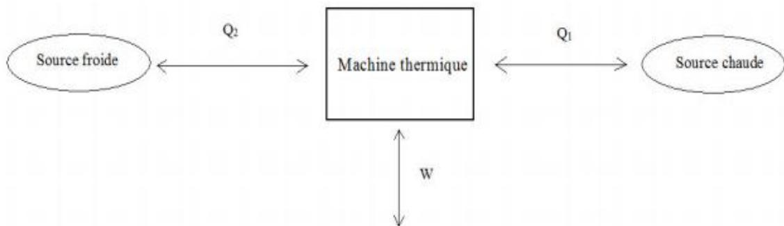
Figure 11: Machine ditherme
