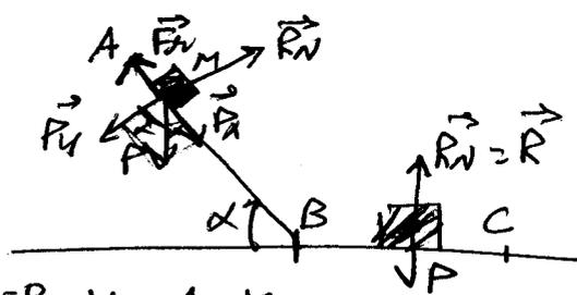
$AB = 1\text{ m}$ ,  $\alpha = 45^\circ$ ,  $V_A = 1\text{ m/s}$
