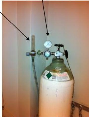
(PHOTO: Gas bottle, regulator and flow meter)
