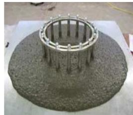
Figure 2 . Essai J-Ring
