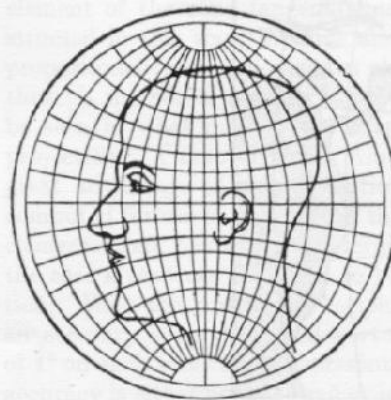
FIG. 45.—Man's head plotted on stereographic projection.
